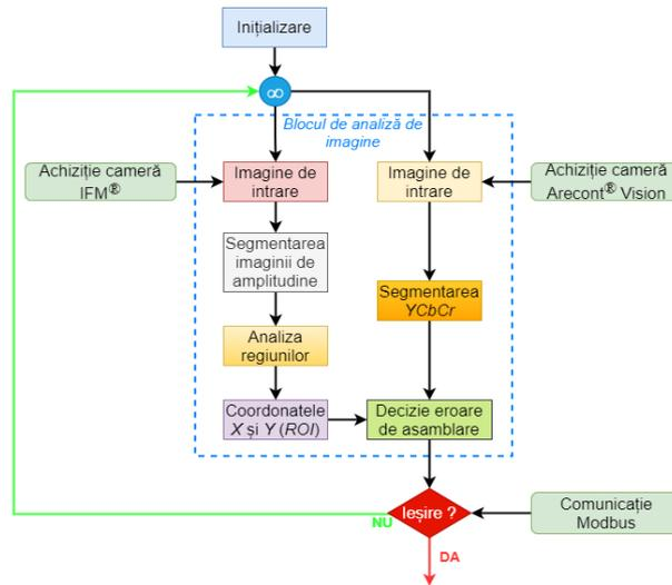
Fig. 3. Functional diagram for the real-time detection error of assembly errors
