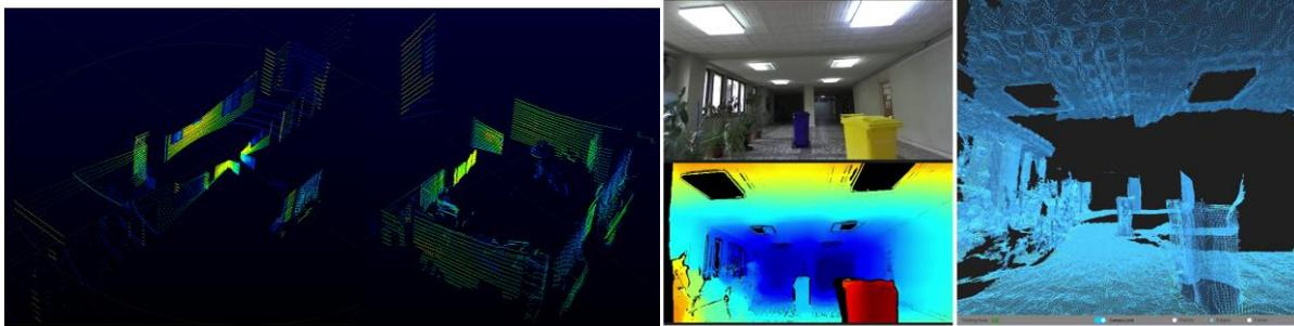
**Switching to one space (left image – hallway) into another space (right image – laboratory). 3D mapping of spaces containing various obstacles using the ZED stereovision system**
