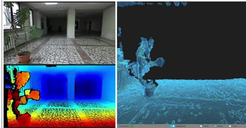
*The 3D space cartography using the stereoscopic video camera ZED*
