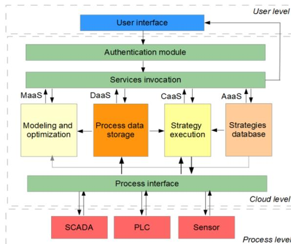
Fig.5 BIB system architecture
