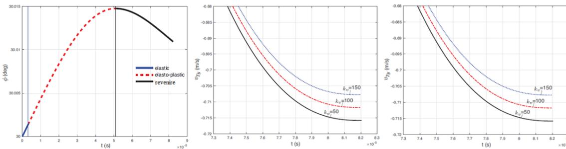
**Impact angle, in degrees, during the impact. Normal bounce rate of the point of impact as a function of the viscous friction coefficient. Angular bounce rate of the bond as a function of viscous friction coefficient.**
