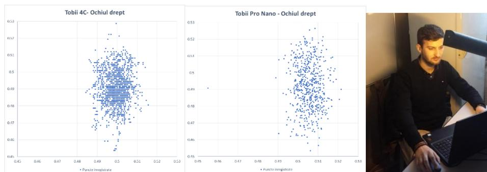
**Comparison of the recordings made for the right eye with the Tobii Eye Tracker 4C device (graph on the left) and Tobii Pro Nano (graph on the right). Tests with artificial light**
