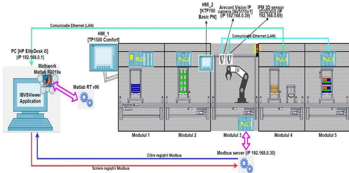
Fig. 2. Schematic of flexible assembly line and computing and communication servers
