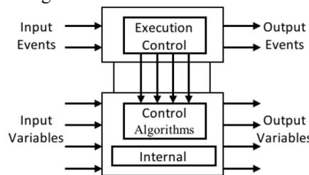
Fig. 4. Representation of a block function according to IEC 61499
