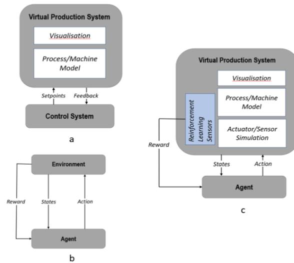
Fig. 7. Comparison between HIL and RL: a) HIL simulation b) RL scheme c) RL scheme on a HIL simulation
