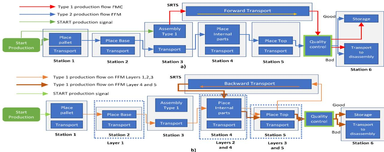
**Figure 3.** Diagram of tasks related to the two production flows: a) Production of Type 1\_single Layers by flexible manufacturing in flow (FFM) and Production of Type 2 by flexible manufacturing in cell (FMC) FFM; b) Production Type 1 - multi\_Layers by manufacturing flow (FFM)
