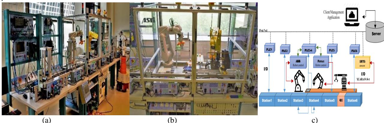
Figure 1. a) SIFF equipped with the robotized systems; b) robot ABB robot (left), robot FANUC si SCARA (right); c) The local control of the workstations and the communication with the Cloud The interaction with the Client-Server/ Management Application
