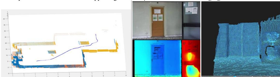
*The trajectory of the mobile platform autonomous movement from the point Ps<sub>2</sub> to the point Pt<sub>2</sub>. The 3D cartography of the access ways using the ZED stereovision system*
